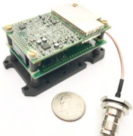
The Inertial Labs **INS-B-OEM** utilizes advanced single antenna GNSS receiver, barometer, 3-axes each of calibrated in full operational temperature range Magnetometers, Advanced MEMS Accelerometers and Gyroscopes to provide accurate Position, Velocity, Heading, Pitch and Roll of the device under measure. **INS-B-OEM** contains Inertial Labs new on-board sensors fusion filter, state of the art navigation and guidance algorithms and calibration software.
